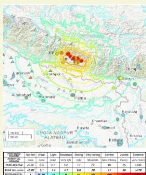
*USGS Earthquake Hazards Program ShakeMap illustrating ground motion and shaking intensity following the initial shock*
