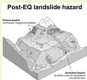
*Earthquakes without Frontiers diagram illustrating primary and secondary earthquake-triggered landslide hazard.*
