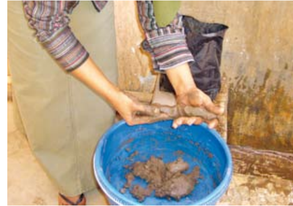
Pic 1. The mud should be mixed with water to form a sticky substance
