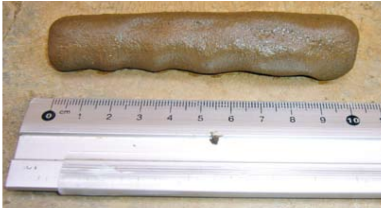
Pic 2. Wet clay rolled into a sausage shape 100 mm in length
