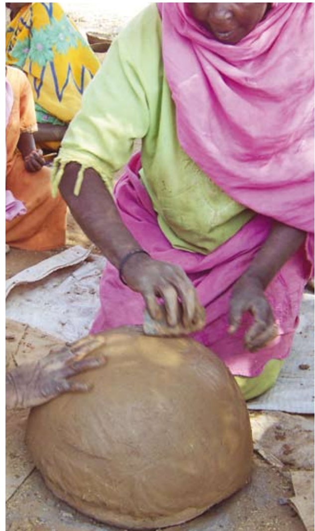
Pic 44. Using water and a stone the surface of the mixture is smoothed.
