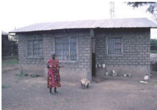
The house in stabilised soil blocks that Mama Susan built
