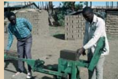
Moulded brick from block press machine, ITDG/ Zul
