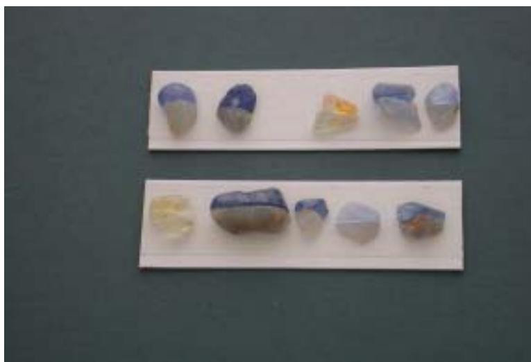
Figure 19: Samples from the Getaheta, Rantapura and Buttala area heat treated at 1800°C in air
