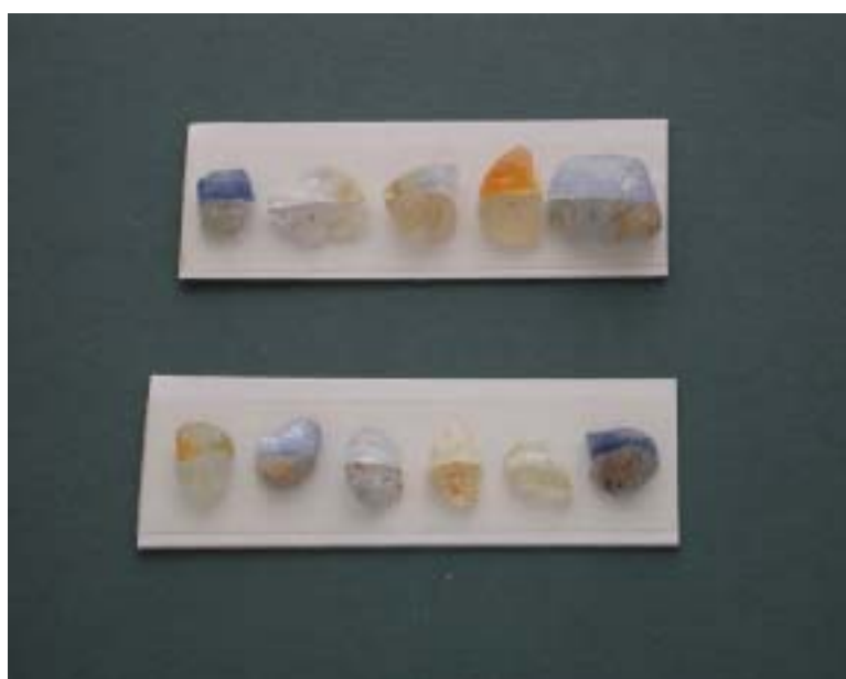
Figure 18: Samples from the Getaheta, Rantapura and Buttala area heat treated at 1800°C in air
