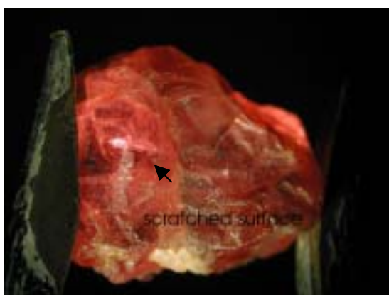
Figure 3: Surface were scratch with a mineral of hardness of 8.5
