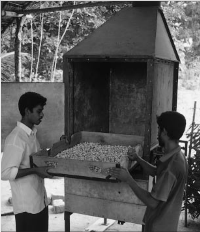
Tray dryer modified for drying cashews
